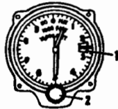
airplane altimeter, reading an indicated altitude of 3000 feet; 1 barometer scale, reading 29.92 inches of mercury; 2 setting knob
